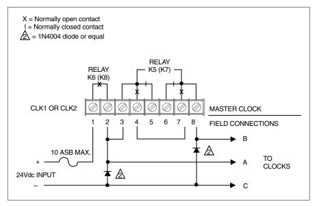
Figure B-18 Three-Wire Minute Impulse (59th Minute) with 12-Hour Correction
